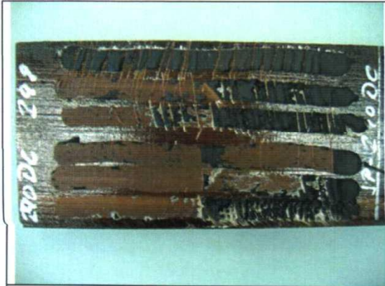
SikaPrimer 290 DC in conjunction with Sikaflex-290 DC + Sikaflex-298
