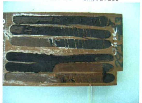
Without Primer in conjunction with Sikaflex-290 DC + Sikaflex-298
